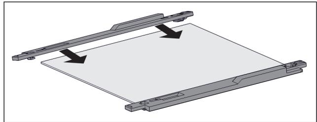
Fig. 61 Glass shelf with retaining part
