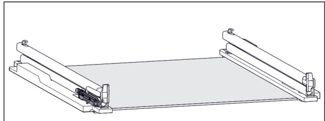
Fig. 62 Damping mechanism
