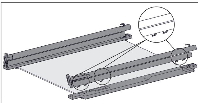
Fig. 59 Glass shelf with rails and retaining parts
